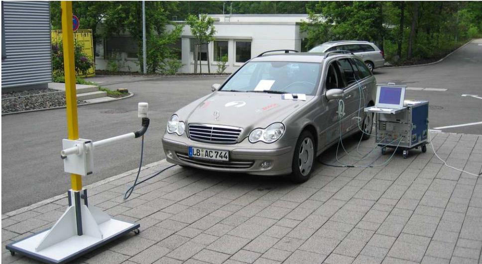
**Figure 5-1: Measurement in the automotive environment with a bi-conical antenna in front of the engine bonnet of a free standing car**
