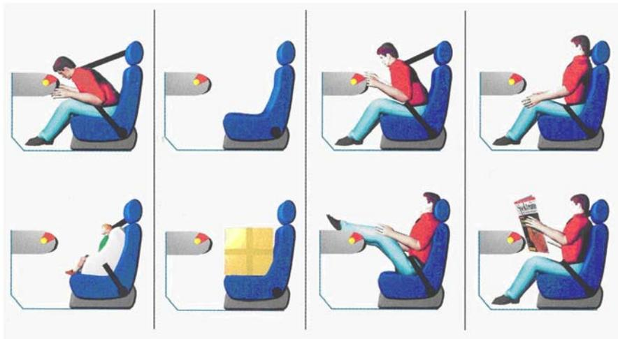
Figure 4-3: Possible cases which have to be covered by occupation sensing (Source: Bosch)
