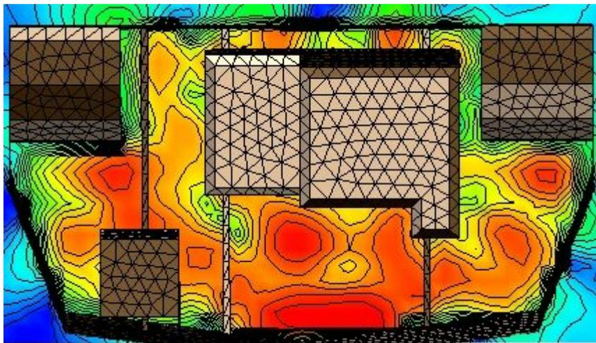
Figure 5-4: Typical distribution of the electrical field of a high frequency signal in the engine compartment
