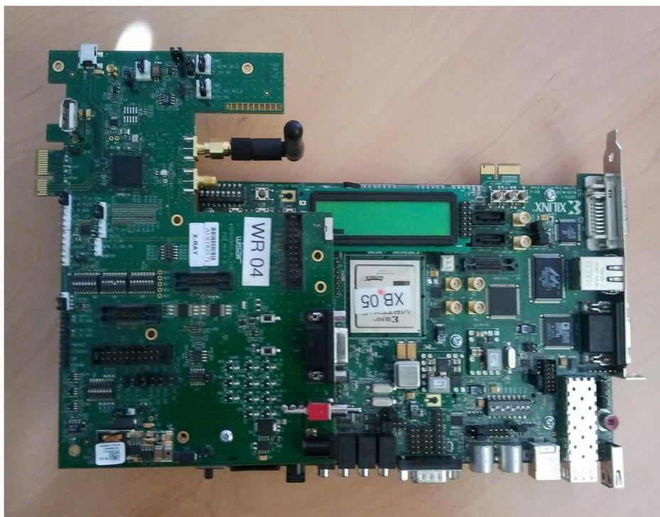
Figure 2: FPGA board Xilinx ML507 and UWB PHY
