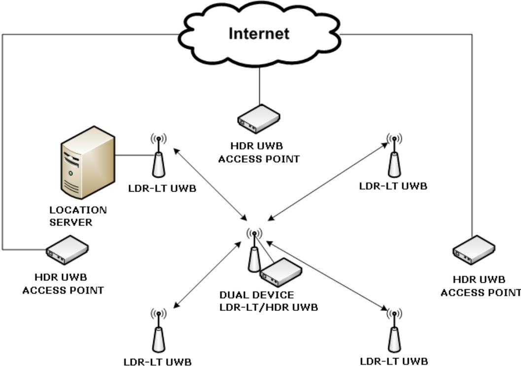
Figure 2-10: Location-aware services demonstrator enhanced with HDR UWB access points
