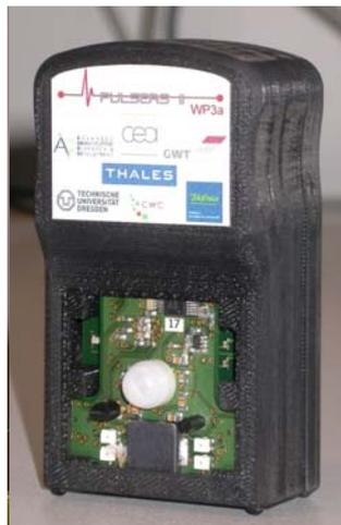
Figure 2-1: Package physical node of the LDR platform
