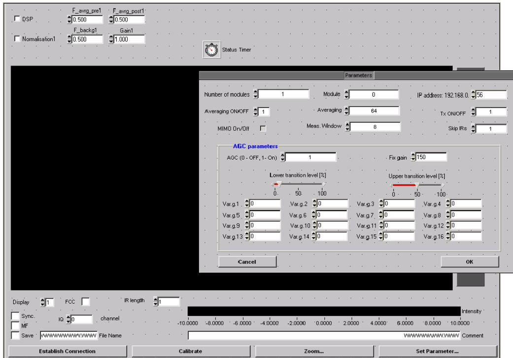
**Figure 3-1: GUI of the sounder program for adjustment of sounder parameters, data monitoring and data recording**
