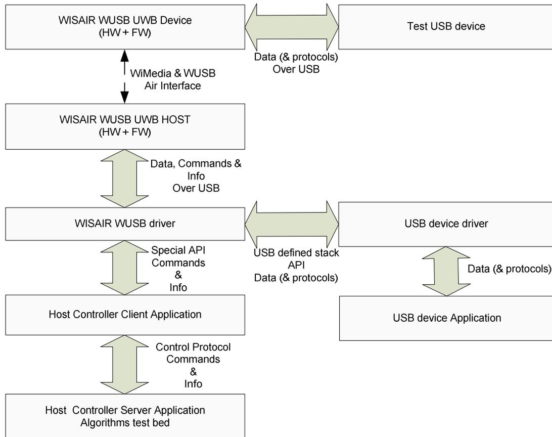
Figure 4-1: Higher Layer Experimental test-bed logical structure
