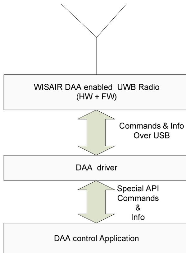
Figure 3-1: DAA Experimental test-bed logical structure
