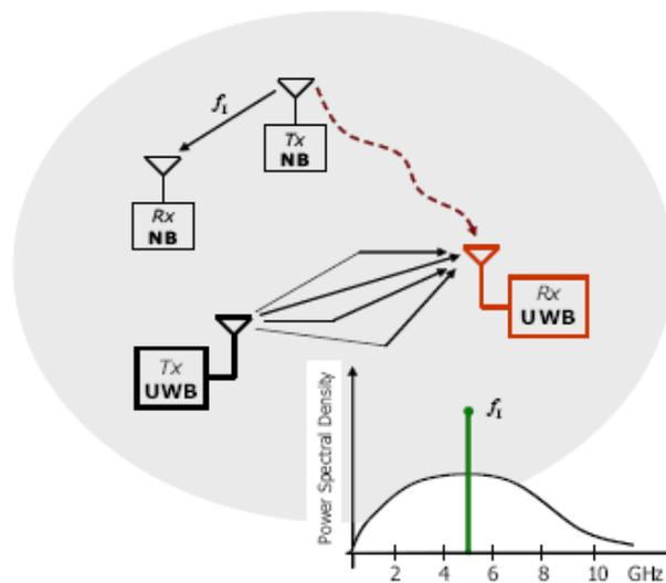
**Figure 4: Coexistence between UWB and narrowband systems.**
